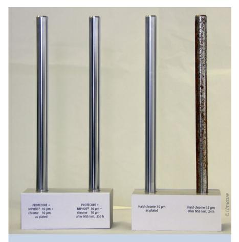
The two-layer system with a 10  $\mu$ m base coat made from nickel-phosphorus alloy and a 10  $\mu$ m chrome layer (left-hand block, right-hand rod) is almost unchanged after 336 hours in the neutral salt spray test (NSS test). In contrast, a 35- $\mu$ m-thick chrome coating shows massive corrosion after 24 hours in the NSS test.
